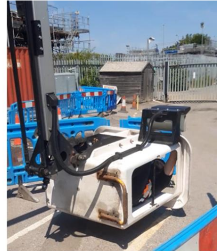
The bucket may return to a full horizontal position. It will not go further than this point.
