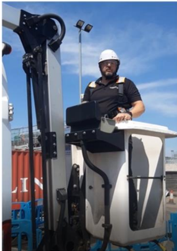
Normal operational position. Operatives should be hooked onto the designated hooking point.
