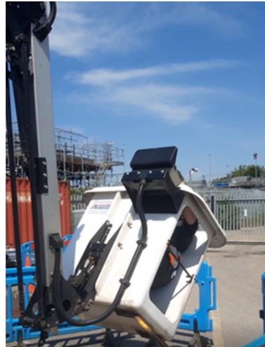
In the event of a hydraulic hose failure, on the bucket MEWP self-leveling mechanism, adopt a crouching position.
